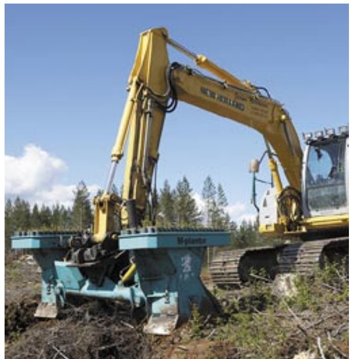
Top Gear: An M-Planter in action in Finland. The machine, excluding reloading, is recorded planting at up to 351 seedlings-per-hour.
