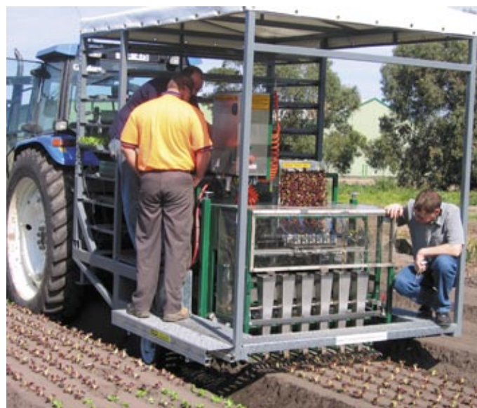
Victorian Solution: Transplant Systems field transplanter can place 7000 seedlings per hour. Those being planted here, however, are lettuce!
